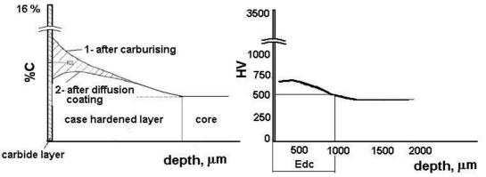
Figure 5. Changes of carbon concentration in the process of duplex layer formation (carburising+diffusion carbide layer formation) and micro-hardness distribution
