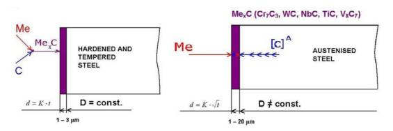
Figure 1. Schematic presentation of the basic difference between the processes of coating and diffusion carbide layer formation
