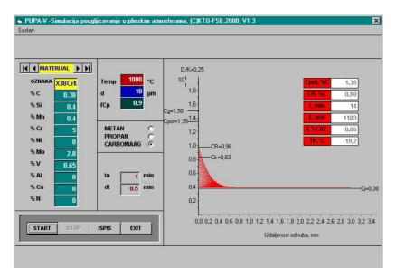
Figure 3. Program interface for the calculation of pre-carburisation parameters for the introducing of carbon required for the formation of a carbide layer of required thickness (10 µm)
