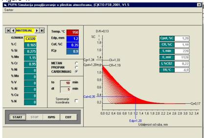
Figure 4. Program interface for the calculation of pre-carburisation parameters for a higher introducing of carbon than required for the formation of a carbide layer
