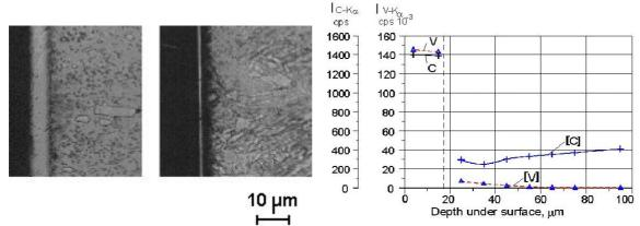
Figure 2. Metallographic cross-sections of different steels vanadised in the same conditions and the qualitative microanalysis of partial de-carburization beneath the carbide layer
